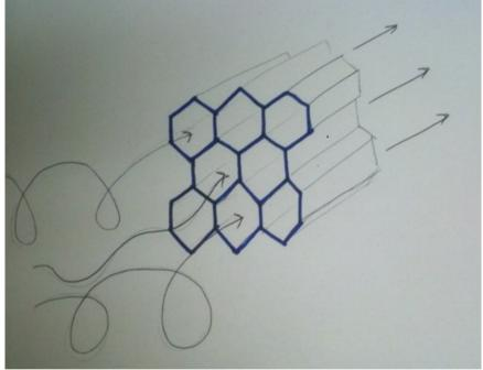
A **flow straightener**, sometimes called a **honeycomb**, is a device used to straighten the air flow in a wind tunnel. It is a passage of ducts, laid along the axis of main air stream to minimize the lateral velocity components caused by swirling motion in the air flow during entry. Bron: Wikipedia
